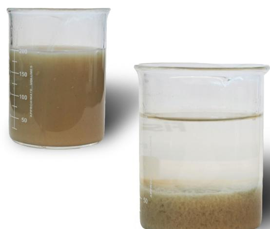
■ Before (left) and after (right) a solids-laden field brine is treated with AES FLOC 4003
