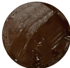
Filtrate (left) and filter cake (right) of EnerREACH system using ENERMUL at 300°F. As part of a properly designed EnerREACH system, ENERMUL provides excellent filtration control and emulsion stability.
