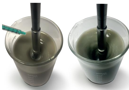
In a lab test, a sample contaminated with shale is treated with KCL SUBSTITUTE (left). As a potassium chloride substitute, KCL SUBSTITUTE efficiently reduces shale hydration (right). Note the larger vortex as reactive clay is inhibited, thinning the fluid sample.
