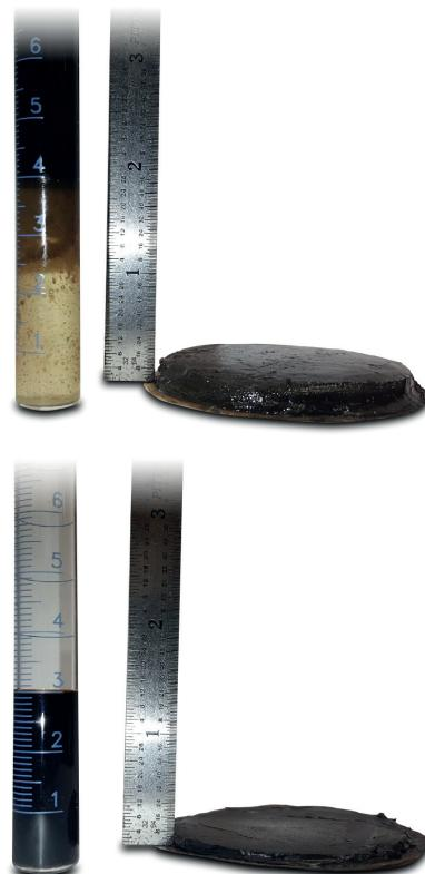
In a lab test, a contaminated 10.5 lbm/gal conventional invert emulsion system demonstrated extremely high HPHT fluid loss and a thickened filter cake (up). A treatment of 4 lb/bbl FLR PLUS, dramatically reduced HPHT fluid loss and cake thickness (down).
